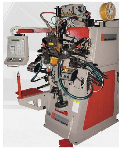
Mark 1 is a heel seat lasting machine by tacks and sides lasting machine by distribution of hot-melt cement for the lasting of footwear for man and lady with any heel height:
